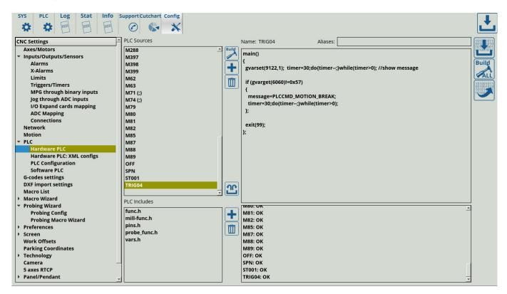
3. In CNC Settings > Probing Wizard > Probing Macro Wizard, click Generate All Probing Macros and Generate PLC Probing procedure M288. Among other settings, this generates the necessary windows for the popup screens of the probe sensor (popup 21 and 22).
