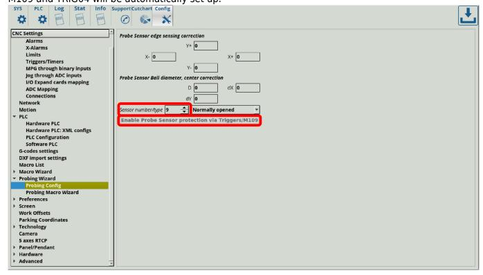
NOTE: The port should always be specified to be normally open in the above window. If the sensor port is normally closed, then it can be inverted in Hardware Settings and set to be "normally open" in the probing config window (with the Rising Edge trigger in Triggers/Timers).
