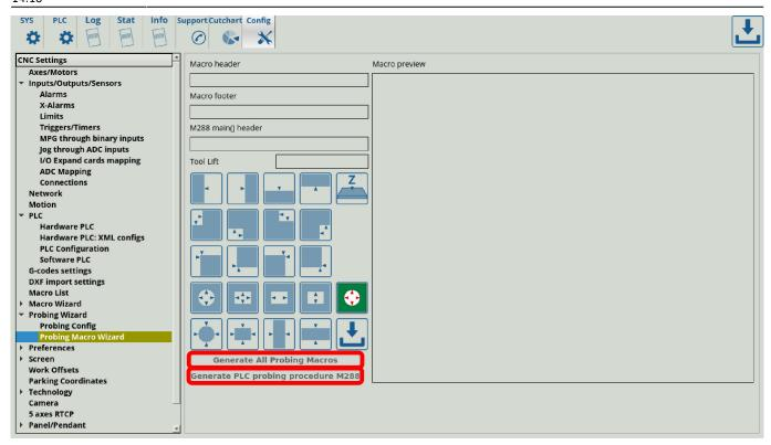
4. After generating the M288 probing procedure, head into CNC Settings > Config > PLC > Hardware PLC and click the Save All, Build All and Send buttons to trigger the PLC disk image reflashing process:
