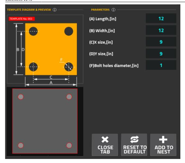
After the operator has selected the necessary custom parameters for the chosen template, it can be added to the CAM editor using the Add to Nest button. Alternatively, the user can reset the parameters of the template to their default values, or close the Shapes tab.
