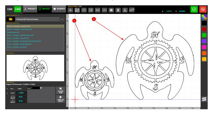
The user can also select whether the dimensions of the DXF file (which is typically unitless when created in a program such as Inkscape, etc) are to be considered to be inches or mm by default.
