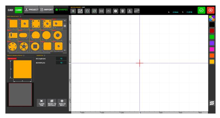
This is the list of 70+ available shapes/parts that are built into myCNC software. These include common shapes such as squares, circles, trapezoids, etc.
