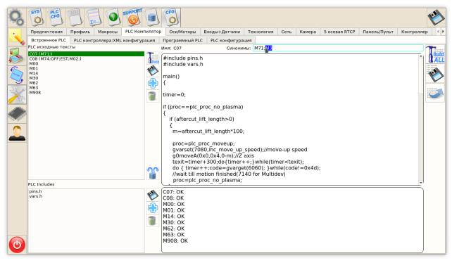
Click in PLC Sources om any other line AND CHECK if in the line with M71 appear M3 in brackets
