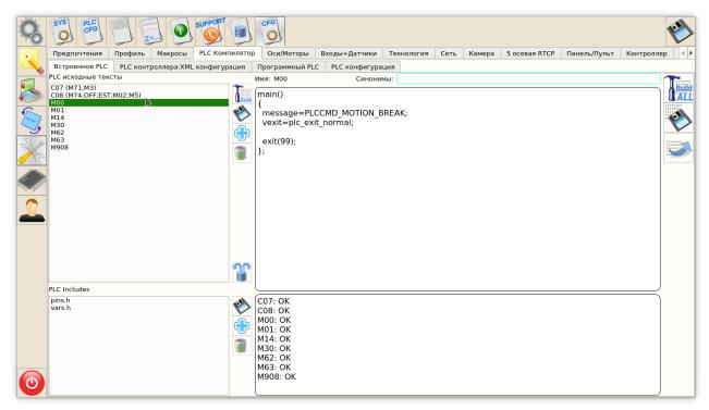
6. Press in series 3 buttons on righ side of PLC Builder - Build All, Save All, Send
