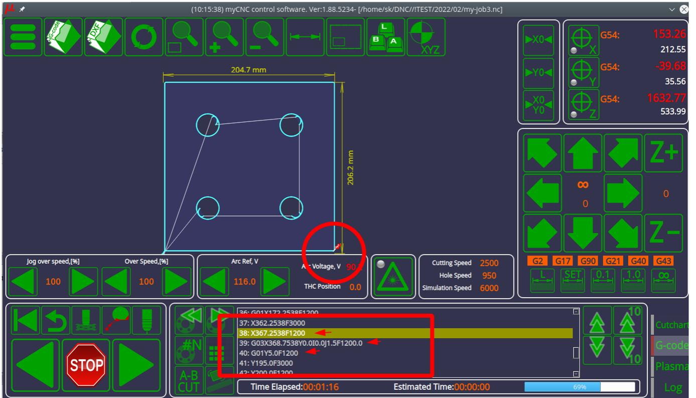
As can be noted from the Path Rules, the example above will have a speed reduction to 40% of the original speed at the arcs on each of the part's corners.
