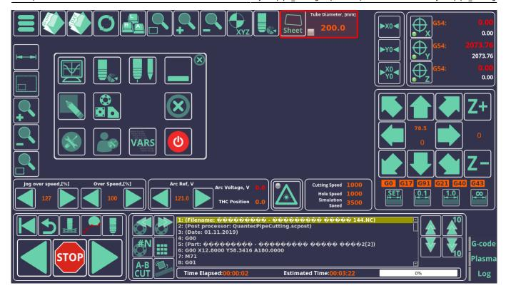
When cutting normally (for applications other then pipe cutting), the Y-axis pulse-per-unit value is taken from the default Axes/Motors field in the myCNC Settings (Settings > Config > Axes/Motors > Pulses per Unit).
