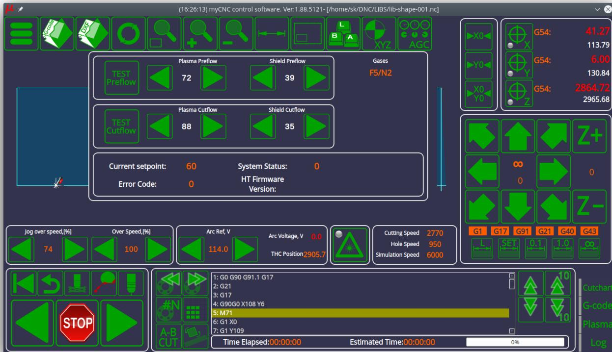
The Automatic Gas Console panel allows to set the preflow and cutflow gas pressures, as well as run the testing procedures on both of those states. The testing software PLCs are available:
